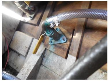
addition the backing blocks and bolts for underwater hard ware is inspected for water tight integrity. Keel bolts, where installed can all contribute water to a bilge and are inspected as well if able to be accessed.
